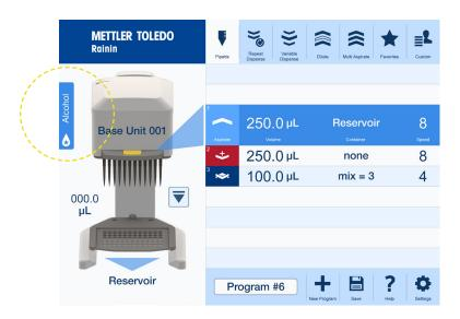
When actively using a liquid class other than the system default, a blue icon with the name of the selected liquid class is shown on the main screen next to the instrument image (see image above).
