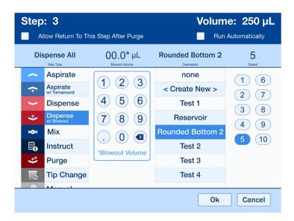
A Tip Change step simply inserts a Tip Load, Tip Eject or full Tip Eject and Load cycle depending on your selections. This allows you to add a tip change anywhere within and is especially useful with long programs that require different types of tips to be used at different times. Note that you can specify whether filter tips should be used, however the instrument will not be able to explicitly verify that the installed tips are filter or non-filter.
