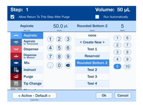
The main difference is that now you can select the type of step you would like to create. Once you have selected the step type, the rest of the pop-up window options will be displayed accordingly. In the case of standard steps — such as Aspirate, Dispense, and Mix — they are identical to what you have used before. Step types available in Custom programs are each a bit different.
