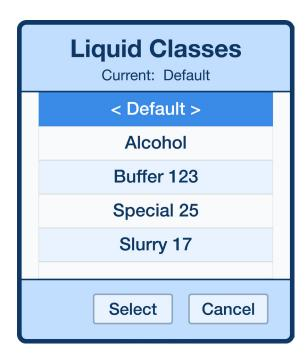
To change the liquid class, simply pressing on the liquid class name opens the separate pop-up window shown above. From here, you can select from any liquid class that has already been created. For more information on creating and using liquid classes, see <u>Section 4.8.6</u>.
