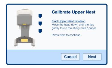
Continue to hold the head in this position and press the NEXT button. The instrument will automatically detect and recalibrate the upper nest position. Once finished, a similar completion message will be displayed.
