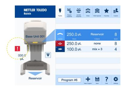
When the reminder elapses, a red exclamation point symbol is shown next to the image of the pipettor on the main screen (see image above). Pressing on this symbol will tell you that it is time for maintenance.
