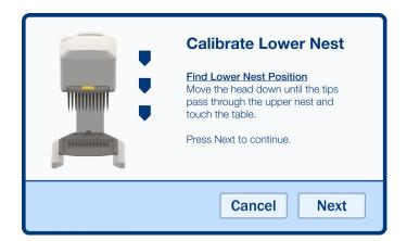
Follow the instructions and lower the head until the tips pass through the upper nest and rest on the table or lower nest position. Continue to hold the head in this position and press the NEXT button. The instrument will automatically detect and re-calibrate the lower nest position. Once this is complete, a new pop-up window will tell you that the nest calibration is complete.
