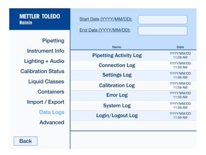
**Pipetting Activity Log** — Displays every program and tip eject/load operation that has been executed using this particular tablet. Each entry contains the type, name, version number, description, date and timestamp of when it was executed. Selecting each entry shows the details of the program or operation. From here you can also modify the date range of entries being displayed as well as sort them by date and time, name, version and type.
