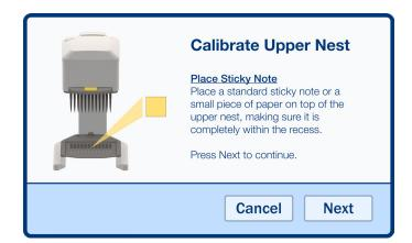
Follow the instructions and place a single sticky note or small piece of paper on the upper nest. Then, bring the head down until the tips are resting on the paper as shown in the pop-up window below. Do not press so hard as to deform the paper.
