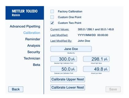
After selecting a Custom Two Point calibration, the screen above is displayed. Here you can enter the desired calibration values along with the subsequent actual values. This will adjust the instrument's calibration curves accordingly. A Custom One Point calibration is functionally the same, but with only a single adjustment point.
