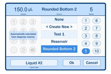
Within this window, you can select the desired container and edit the speed. However, the aspirate volume is calculated directly from the dispense values and is therefore not editable here.
