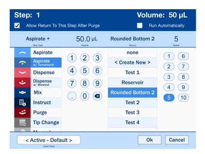
When selecting the Instructions step, you are asked to provide the headline and instructions to be displayed. Once an Instructions step has been created, the headline of the instructions will be shown in the step on the main screen. In this case the volume and speed columns will be left blank.
