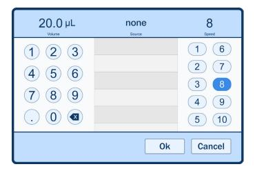
Pressing on the dispense or add mix step will bring up pop-up windows that are also identical to the simple Pipette with Mix function. Except that the dispense volume is not editable because it is calculated automatically from the total aspirate volume.
