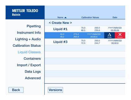
To modify or remove a liquid class that has already been created, swipe that row to the left to reveal the Modify and Reveal buttons (see image above). Once you select a liquid class, you can also press the Versions button which will display all the previously saved iterations of that liquid class. Here, you can also view and export detailed specifications of each version.
