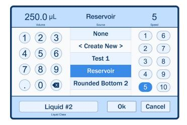
Within this pop-up window you can edit the volume, select the desired container, edit the speed and select a liquid class. To edit the volume, simply use the keypad to enter in the desired volume in  $\mu L$ . From the list of containers, you can select any of the pre-existing containers, select none or choose to create a new one. See Section 4.6 for details on creating a new container. Note that this is the container that liquid will be aspirated from.
